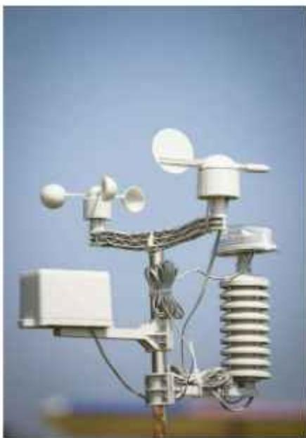
QES-WMS-01 Weather Stations are highly sophisticated monitoring & logging of intrinsic weather conditions like temperature, barometric pressure, wind direction, wind speed, wind chill and other optional parameters according to your requirements.
