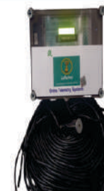
Piezo Meter With Telemetry System
